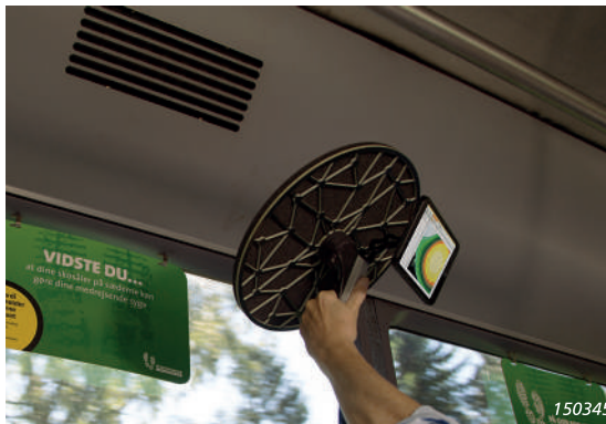
Fig. 4 Left: Array WA-1764-W-001 with reflective plate for use in beamforming measurements Right: Without reflective plate for use in acoustic holography measurements
