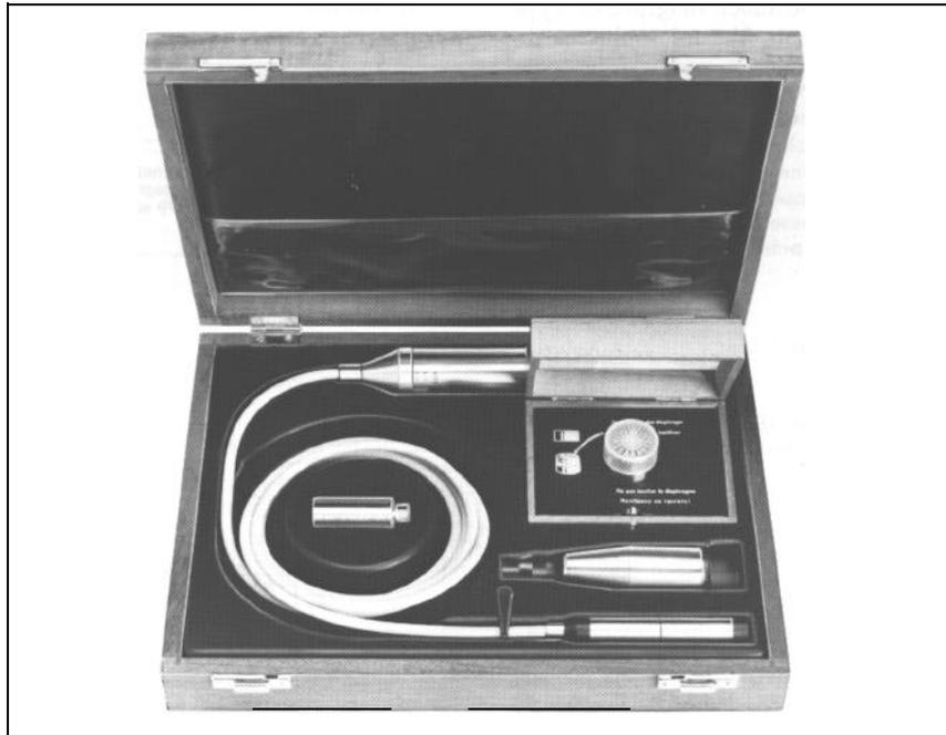
Brüel & Kjær has developed the 1" Condenser Microphone Type 4179 and Microphone Preamplifier Type 2660 system for measuring ultra-low sound pressure levels. High-quality, conventional 1" condenser microphones, such as B&K Types 4144 and 4145, and half-inch diameter Types 4165 and 4166, provide for the majority of noise measurements to IEC, ISO
