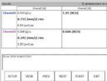
Two-channel real overall measurements (bandpass/BCU)
