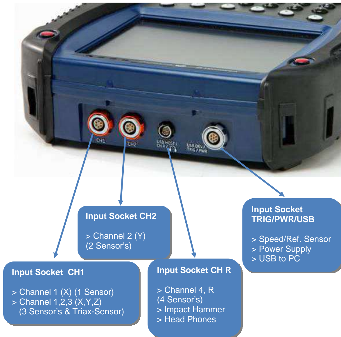
Figure 1: Overview Backplane with explanation – VP-80 (shown) identical to VT-80
