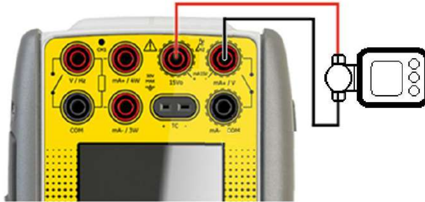
Figure 6-1 Positioner Connection with Internal Loop Supply
