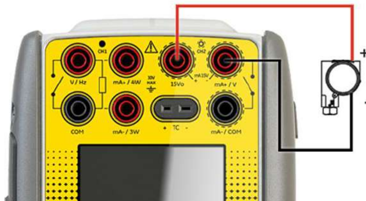
Figure 3-1 Connection with Internal Loop Supply
