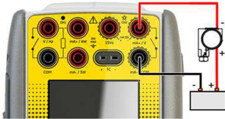
Figure 2-1 Connection with External Loop Supply
